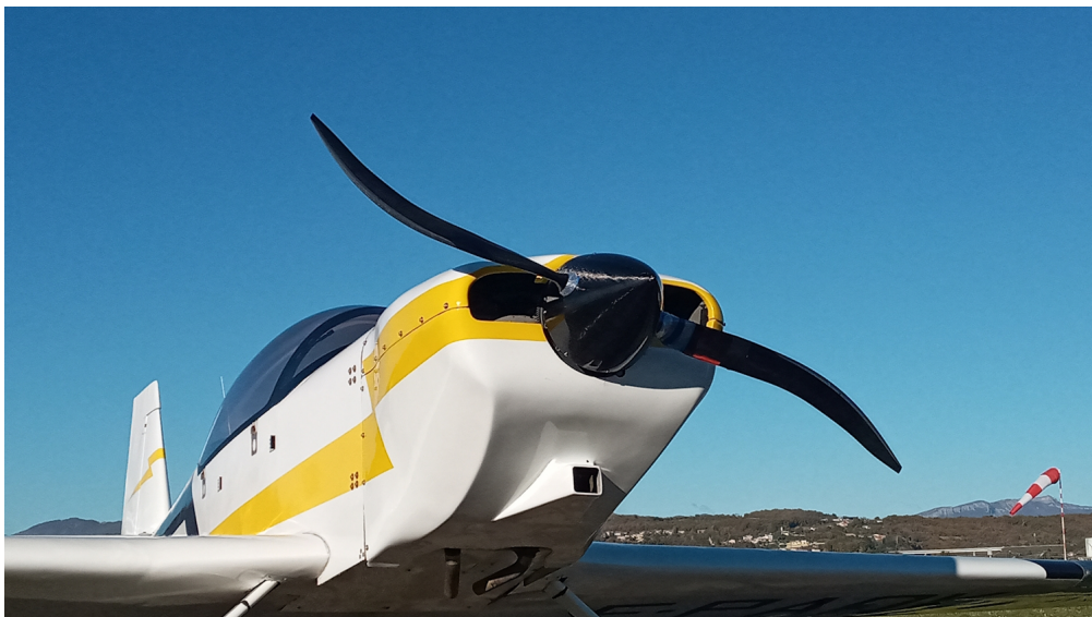
PENA Bilouis – Lycoming O-360 (180 hp) – 2-blade ASCALON ground-adjustable-pitch propeller, showing a strong ESR effect on a direct-drive installation.
