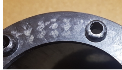
E-Props carbon drive lugs integrated to the spacer
